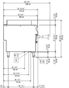
EQ = Equipotential screwG = Gas connection
